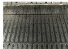
Vertical groove guide gas platform, make paper surface more smooth
