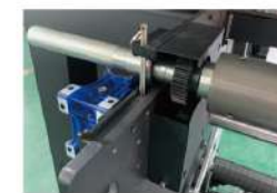
Inflatable shaft upgrade is sliding type, convenient materials up and down
