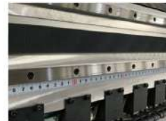
Wider and thicker girder with THK silent double guide rails
