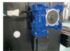
Feeding adopt servo motor, make the paper more stable and more accurate
